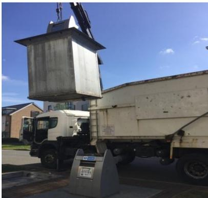
iv Underground bin being collected by crane operated vehicle
