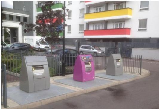
iii Fully underground bins with small visible receptacle
